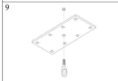
Insert the  $\frac{3}{4}$ " Eye Bolt (15) and secure with the  $\frac{3}{4}$ " Nylon Lock Nut (12).
