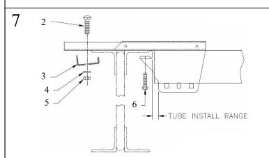
When completely installed, each Jaw Clamp should be attached to the joist with the heel clip (3) as well as the self locking bolt (6). The Main Tube (11) should be set within the specified range as shown above. **Note:** Be sure to clear the edge when attaching bolts and heel clip to a cold formed joist.
