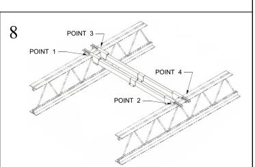
Repeat steps 3-7 for the second Main Tube in roof deck opening above Point 3 and Point 4. Make sure the Main Tubes and Jaw Clamps are aligned and tight.
