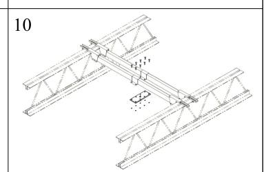
Align the Fall Protection Bracket Clamps on each tube with each other. Insert Carriage Bolts (9)(qty:8) into the Fall Protection Bracket Clamps from the top down. Install the Fall Protection Anchor Plate (13) and secure with the Nylon Lock Nuts (14). Tighten all connections.
