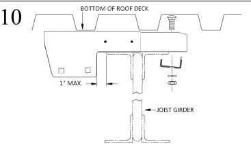
Slide Girder Clamp (1) over joist girder and below roof deck at location directly across from corresponding T-Bracket. Attach this Girder Clamp with Heel Clip (3) and tighten. Make sure the Girder Clamp is no more than 1" from joist as shown. Repeat for each Girder Clamp.
