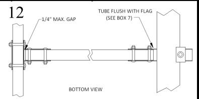
Insert Cross Tube into wings of T-Bracket and Girder Clamp as shown. Be sure tube is within <sup>1</sup>/<sub>4</sub>" of the back of the T-Brackets and Flush with the back of the Girder Clamp flag. Secure with bolts and locknuts. Repeat for each desired Cross Tube. Tighten everything.
