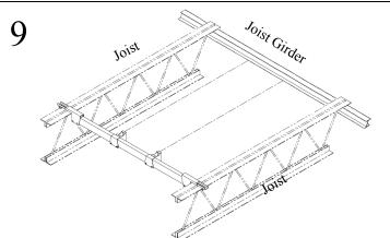
Identify four points that form a rectangle on the Main Tube and Joist Girder. This is where the T-Brackets and Girder Clamps will be installed. Slide T-Brackets to desired locations. Tighten bolts.
