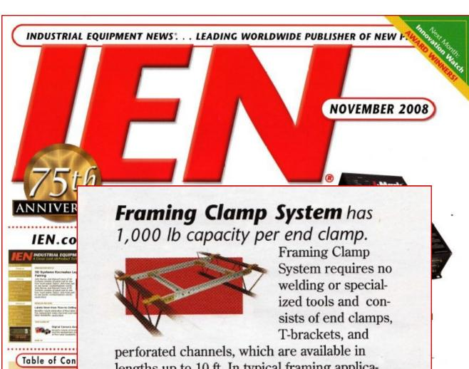
perforated channels, which are available in lengths up to 10 ft. In typical framing application, 4 end clamps are attached to 2 parallel bar joists or beams, and each end clamp occupies 1-1/4 x 3 in. space between joists. System is designed for installing HVAC equipment, exhaust fans, vents, and skylights; framing roof openings; and supporting loads above or below roof decks. **Chicago Clamp Co.**; 866-633-6798 708-343-8311; Tech Contact: Kevin Barry
